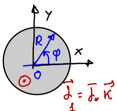
$$\vec{B}_1 = \begin{cases} \vec{B}_{1i} = \frac{\mu_0 J_0}{2} \rho \vec{u}_\phi & \text{si } 0 < \rho \leq R \\ \vec{B}_{1e} = \frac{\mu_0 J_0 R^2}{2\rho} \vec{u}_\phi & \text{si } \rho > R \end{cases}$$
