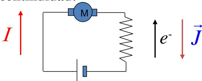
$$\left. \begin{aligned} \oint_S \vec{J} \cdot d\vec{S} = I' = -\frac{dQ}{dt} \\ \int_v \nabla \cdot \vec{J} dv = -\frac{d}{dt} \int_v \rho dv \end{aligned} \right\} \rightarrow \nabla \cdot \vec{J} + \frac{\partial \rho}{\partial t} = 0$$
