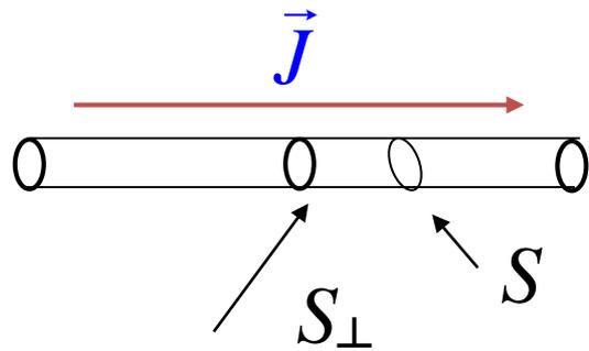
$$I = \int_{S_{\perp}} \vec{J} \cdot d\vec{S}_{\perp} = \int_S \vec{J} \cdot d\vec{S} = \int_S q_e \frac{dN}{dV} \langle \vec{v} \rangle \cdot d\vec{S} = q_e \frac{dN}{dV} v S_{\perp} = q_e \frac{dN}{S_{\perp} dl} \frac{dl}{dt} S_{\perp} = \frac{q_e dN}{dt} = \frac{dq}{dt} \quad (\text{en } A = C/s)$$
