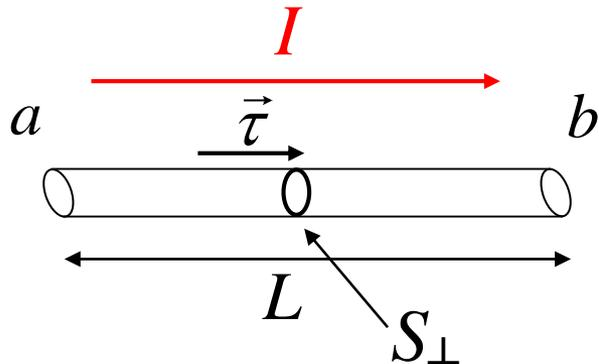
$$I = \int_{S_{\perp}} \vec{J} \cdot d\vec{S}_{\perp} = J S_{\perp} \quad \vec{J} = \frac{I}{S_{\perp}} \vec{\tau}$$
