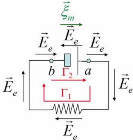
$$\left\{ \begin{array}{l} \oint \vec{E}_e \cdot d\vec{l} = 0 \\ \int_{a \Gamma_1}^b \vec{E}_e \cdot d\vec{l}_{ab} + \int_{b \Gamma_2}^a \left( \frac{\vec{J}}{\sigma_c} - \vec{E}' \right) \cdot d\vec{l}_{ba} = 0 \\ (V_a - V_b) + Ir - \varepsilon = 0 \end{array} \right.$$
