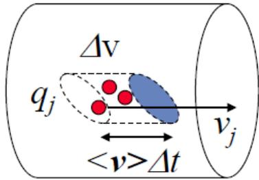
$$\frac{\delta W}{dt dv} = \frac{\sum_{j=1}^{j=dN, en dv} q_j \vec{E}(\vec{r}_j) \cdot \vec{d\vec{r}}_j}{dt dv} = \frac{dP}{dv} \quad (W / m^3)$$
