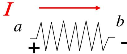
$$V_a - V_b = I \int_a^b \frac{dl}{S_{\perp} \sigma_c} = I R, \quad 1 \Omega = \frac{1V}{1A}$$
