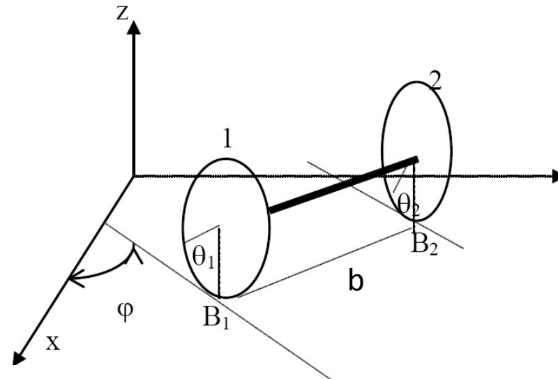
$$\bar{v}_{B2} = 0 \Rightarrow \begin{cases} \frac{d}{dt}(x_1 - b \sin \varphi) - R\dot{\theta}_2 \cos \varphi = 0 \\ \frac{d}{dt}(y_1 + b \cos \varphi) - R\dot{\theta}_2 \sin \varphi = 0 \end{cases}$$
