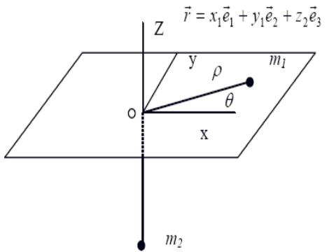
$$\text{ligadura} : \phi = \sqrt{x_1^2 + y_1^2} - z_2 - L \equiv \rho - z_2 - L = 0$$
