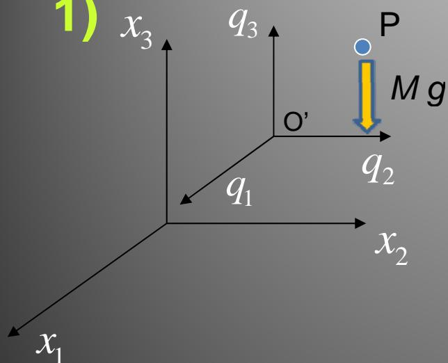
$$\vec{r}_{o'}(t) = x_{o'}(t)\vec{e}_1 + y_{o'}(t)\vec{e}_2 + z_{o'}(t)\vec{e}_3,$$
