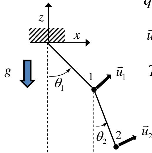
$$q = \theta_1, \theta_2, T = \frac{M}{2} \left( \vec{v}_1^2 + \vec{v}_2^2 \right), \quad \vec{v}_1^2 = \ell^2 \dot{\theta}_1^2, \quad \vec{v}_2 = \ell \dot{\theta}_1 \vec{u}_1 + \ell \dot{\theta}_2 \vec{u}_2,$$
