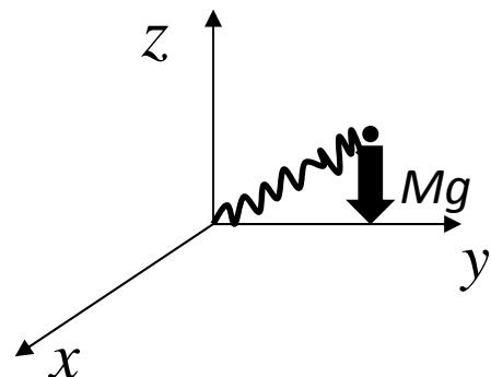
$$\frac{\partial L}{\partial t} = 0, \quad B_1 = 0 \quad \rightarrow \quad E = T + U = \text{const.}$$
