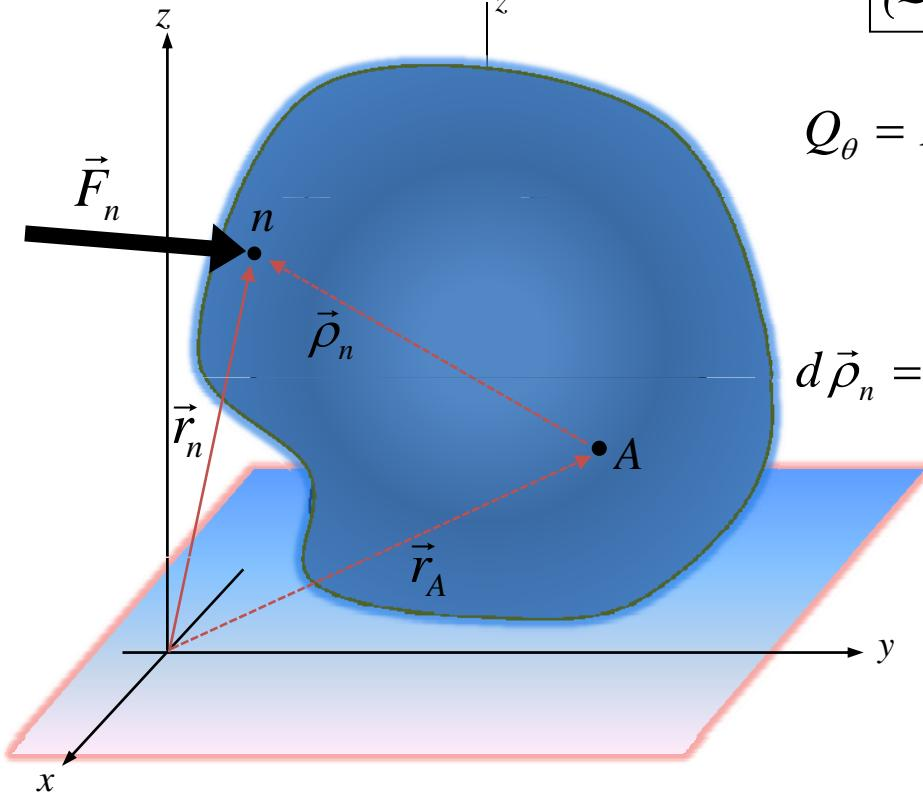
$$Q_\alpha = \vec{f} \cdot \vec{a}_\alpha = \vec{f} \cdot \frac{\partial \vec{r}}{\partial q_\alpha} = \vec{F}_n \cdot \frac{\partial \vec{r}_n}{\partial q_\alpha},$$
