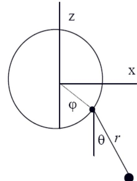
$$T(r, \theta, \dot{r}, \dot{\theta}, t) = \frac{1}{2}m(\dot{x}^2 + \dot{z}^2) = \frac{1}{2}m((R\omega \cos \varphi + \dot{r} \sin \theta + r \dot{\theta} \cos \theta)^2 + \\ + (R\omega \sin \varphi - \dot{r} \cos \theta + r \dot{\theta} \sin \theta)^2),$$
