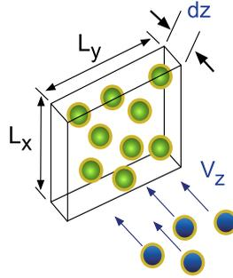
**Figure 2.5.** Target particles within  $L_x \times L_y \times dz$ .
