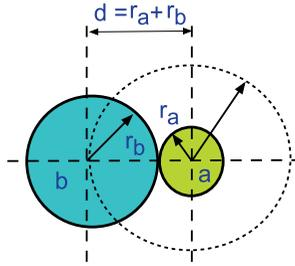
**Figure 2.3.** The area within the dotted circle is the total cross section  $\sigma_{ab}$  for colliding particles.
