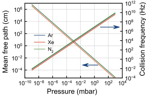
**Figure 2.6.** The mean free path  $\lambda_c$  (left) and the collision frequency  $\nu_c$  (right) as a function of the gas pressure  $p_a$  calculated using the values of table 2.1.
