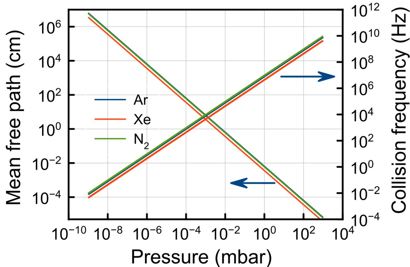
For collisions between gas particles (“aa”) in thermal equilibrium using the ideal gas equation  $p = n_a k_B T$
