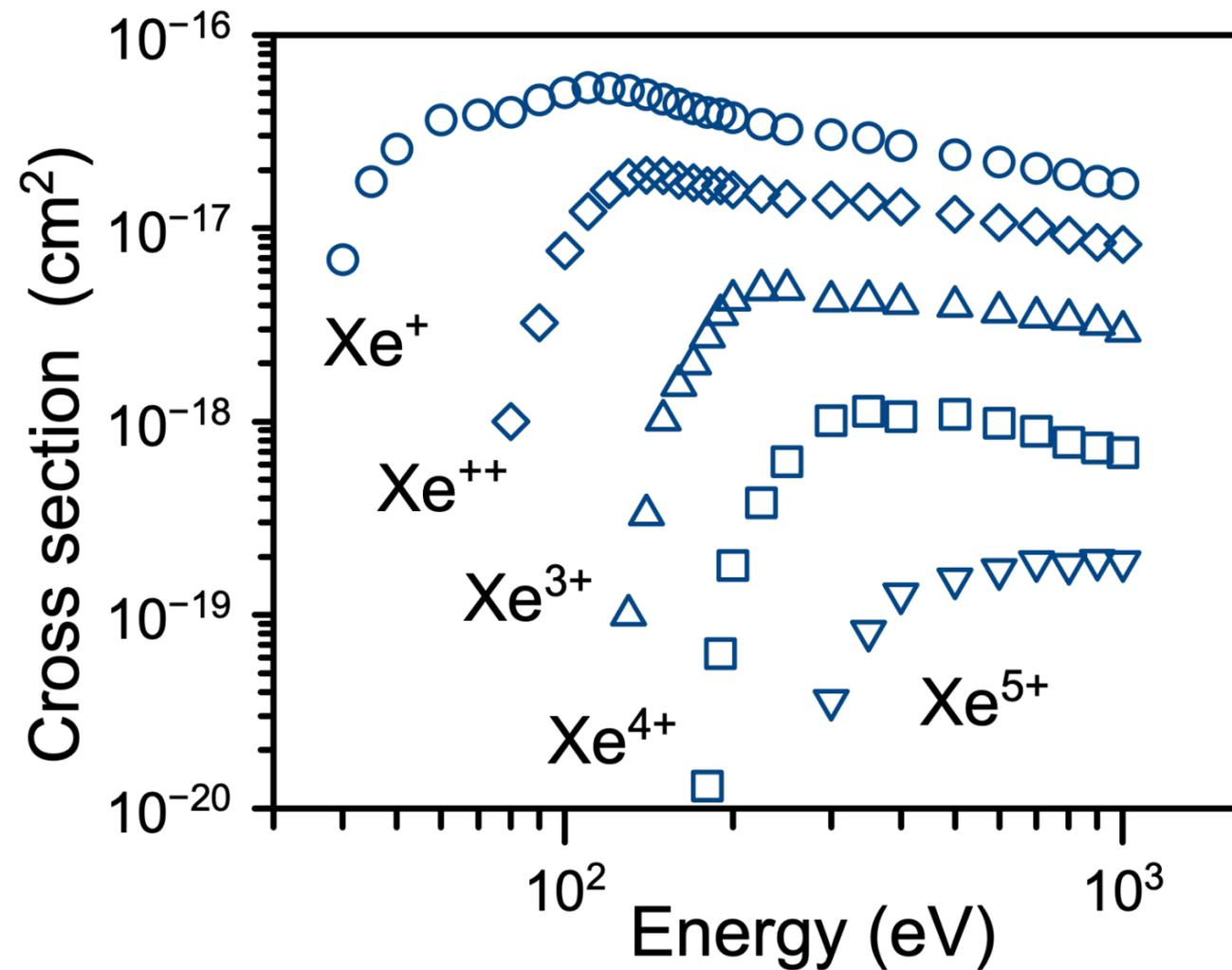
The total ionization cross section of Xenon by electron impact  $X_e + e \rightarrow X_e^n + ne$  of interest in plasma propulsion as this gas is used as propellant due to its low ionization energy.
