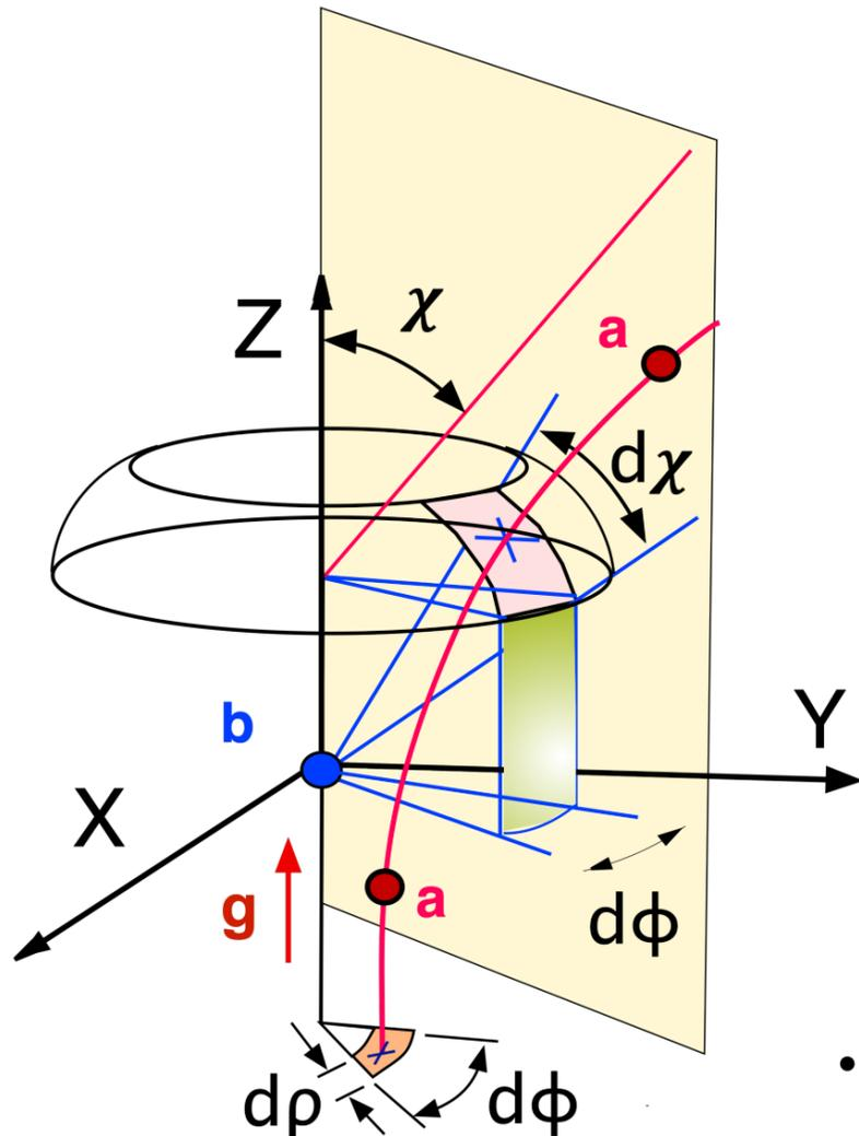
The  $\dot{Q}_a = \Gamma_a dS$  particles "a" (by time unit) crossing section  $dS = (\rho d\phi) \times d\rho$  with velocity  $\mathbf{g} = \mathbf{v}_a - \mathbf{v}_b$
