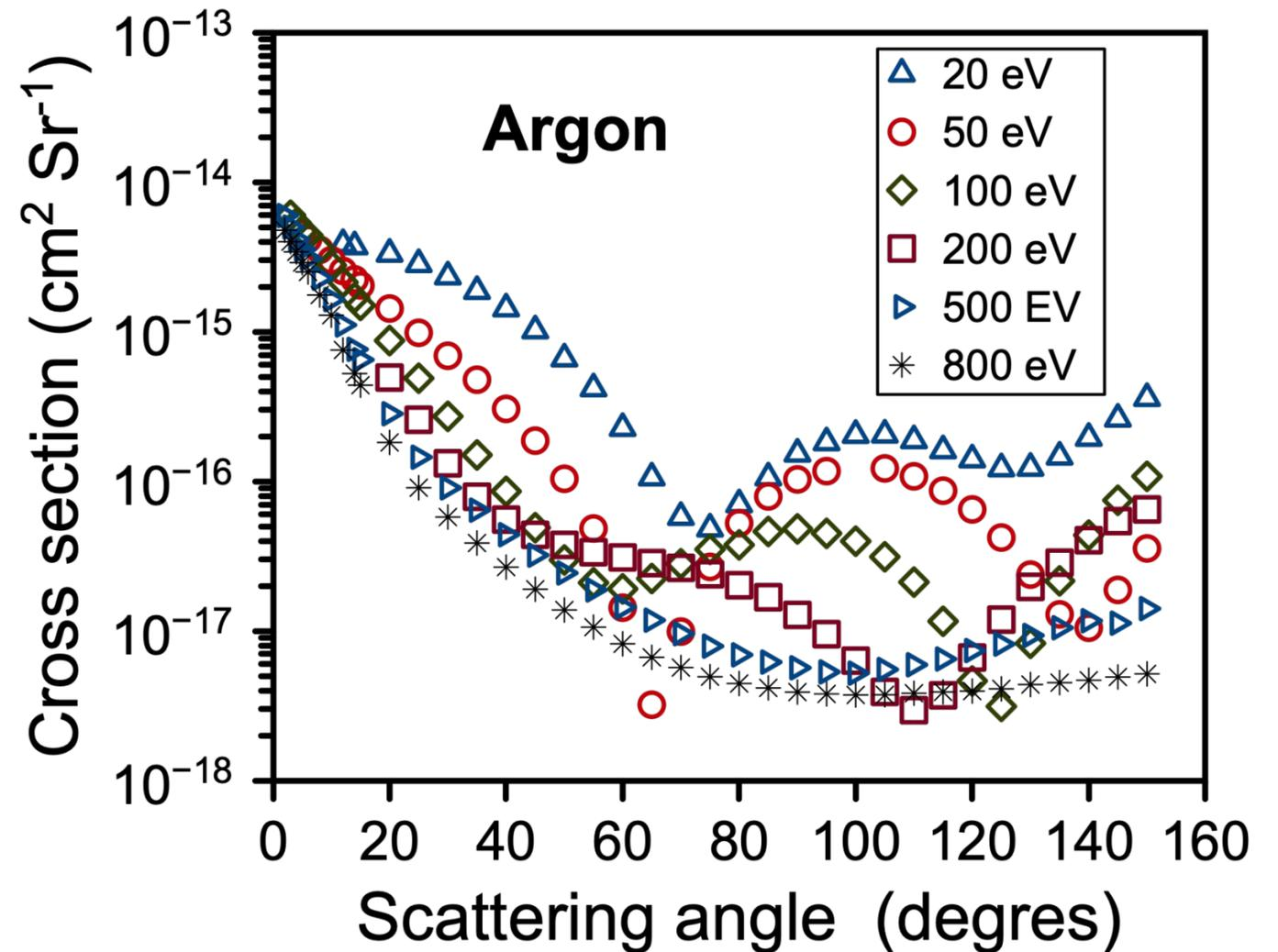
The differential cross section of elastic scattering  $Ar + e \rightarrow Ar + e$  of electrons by Argon atoms. The values depends on the energy and the angle of incidence of the electron.
