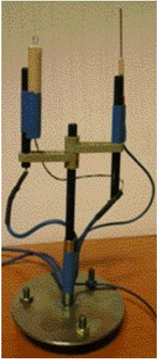
The support for the collecting and emissive Langmuir probes in the plasma chamber
