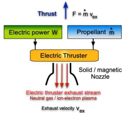
**Figure 2.** The scheme of a EP system with electric power  $W$  and propellant mass flow rate  $\dot{m}$  consumption.
