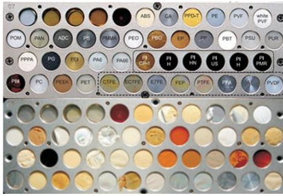
FIGURE 2. Pre-flight and post-flight photograph of the MISSE 2 PEACE polymers experiment tray [10].
