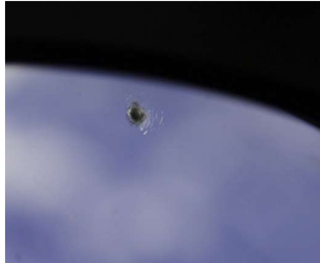
Micrometeoroid impact on window #7 of ISS Zvezda service module, source NASA.
