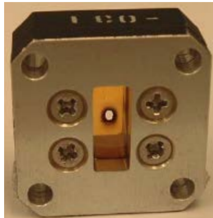
Harmful effects of secondary electron multiplication (multipactor) within RF communication equipment. Photographs courtesy of ESA.
